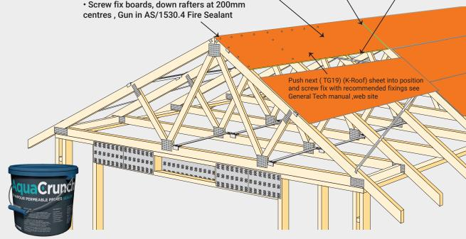
FIRECRUNCH GENERIC ROOF COMPONENTS DIAGRAM to meet AS /3959, roof design . Methods will vary according to individual designs
