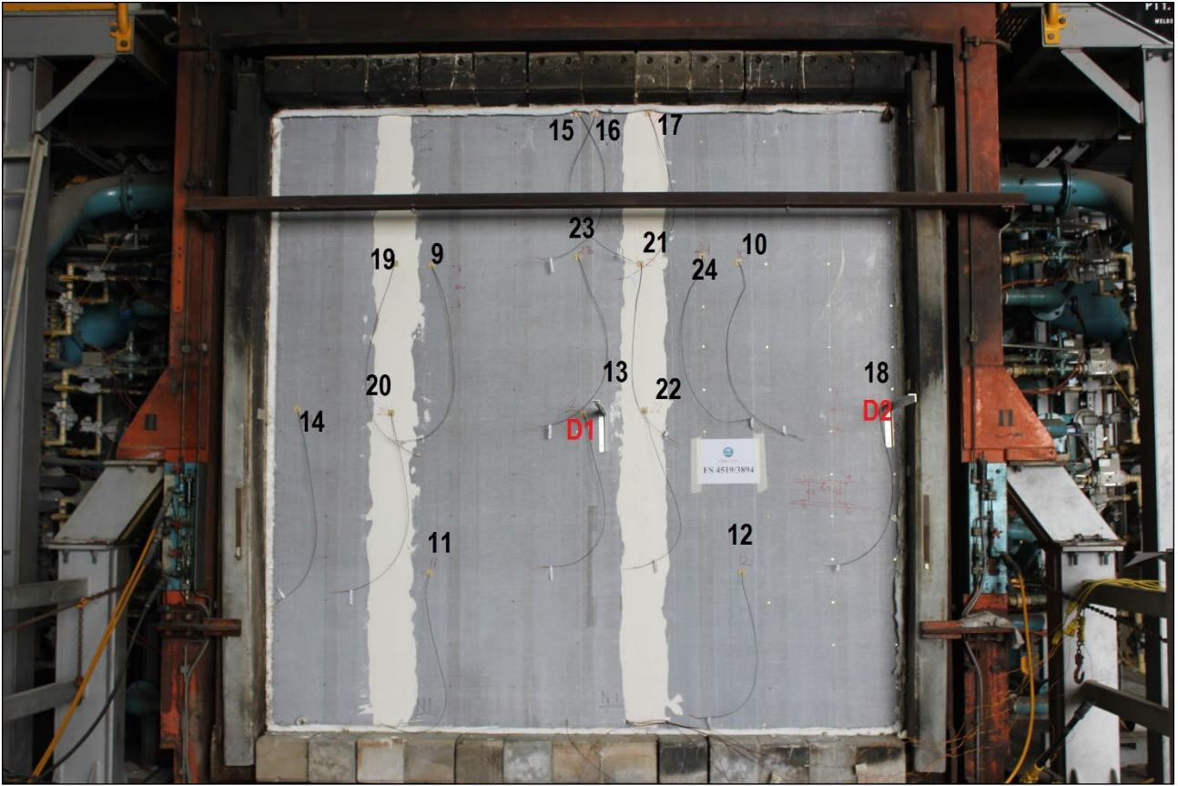
Figure A1: Unexposed face of test specimen detailing external face thermocouple locations
