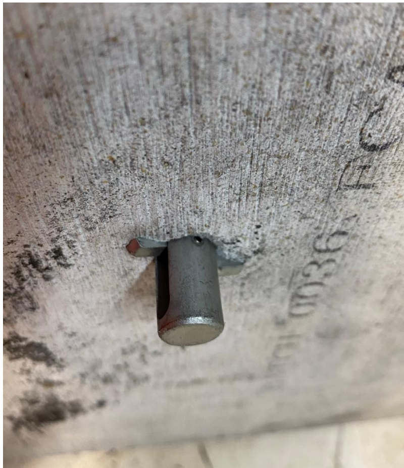
Figure 6 Typical failure of single bolt test
