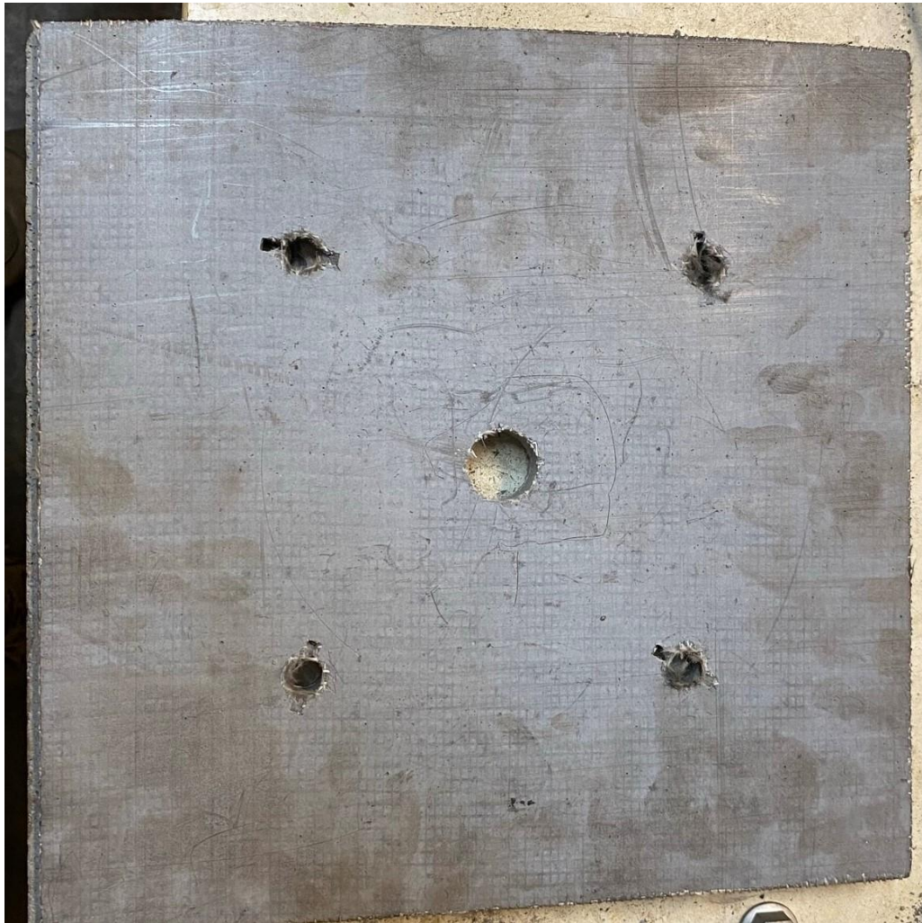
Figure 7 Typical failure of four bolt test (Rough Side up)
