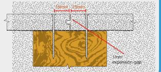
FILL fire /weather sealant Bostik Fire Ban or other AS1530.4 product to the grooved edge of board, before the next sheet is positioned and fixed and ensure the joint is adequately filled.
