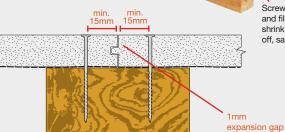
Screw fix 50mm from corners and fill screw holes with non shrink 2 pack epoxy and screed off, sand when dry
