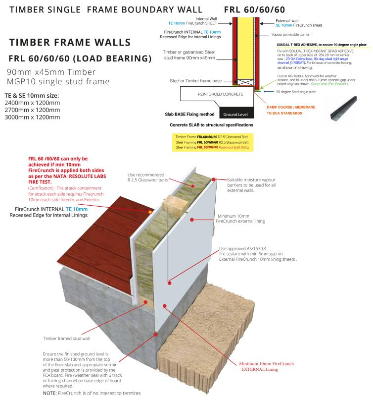
plaster board 13mm can be used for interior walls in free standing homes, However FireCrunch CSIRO Certificates can not be used and a separate assessment is required by a fire engineer as if the test materials are changed it invalidates the certificates.
