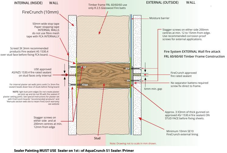
2nd : Dulux Precision Maximum Strength Adhesion Primer + 3rd : Dulux top coat colour https://firecrunch.com.au/wp-content/uploads/2020/12/02\_01\_FireCrunch-Sealer\_Prime-and-Painting-Manual.pdf
