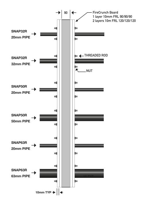
The FireCrunch 10mm TEST and assessment for fire seperation walls based on the CSIRO, NATA Fire Test on a COLD ROLLED STEEL FRAME 1.15 BMT (90mm cavity using Rockwall fire batts). This is a DTS system .
