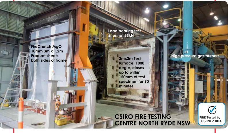
Tests are rated in "load bearing" which are shown in three figures ,and tests in Non load bearing shown as 2 firgures. IE **FRL ( Fire Resistance Level) Load bearing**
