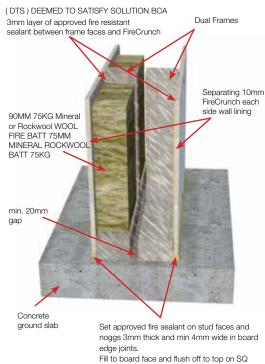
edge board and to top level of recess in recessed edge board internally where plaster set is to be applied later.
